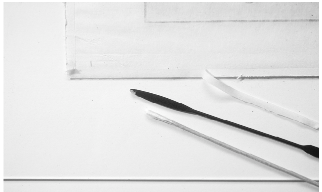
Fig. 8. Detachment of the paper strip and removal of adhesive residues
