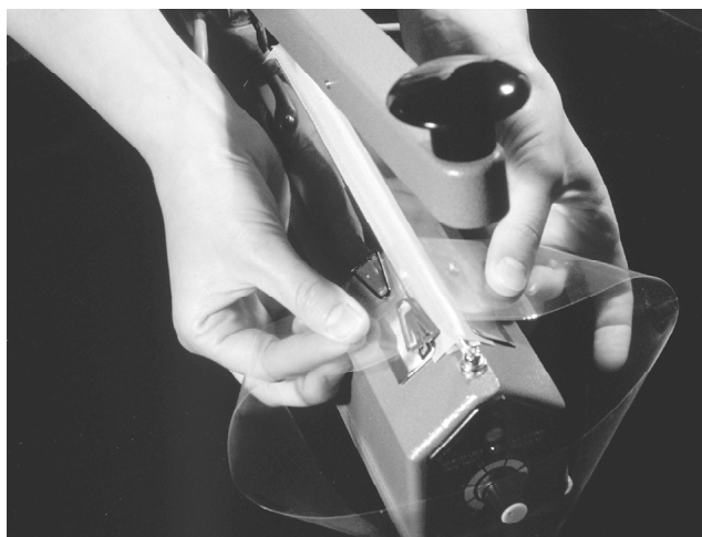
Fig. 3. Slide the strapping off of the cover. Set the dial on the Thermo Impulse Sealer to 3. Place the strapping between the seal bars of the Thermo Impulse Sealer.
