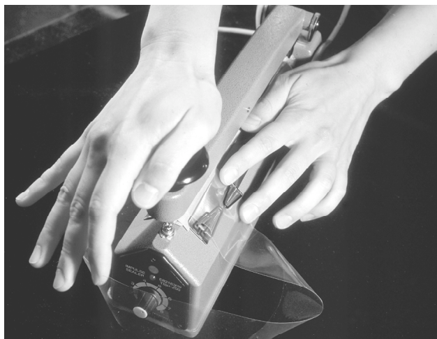
Fig. 4. Press down on the lever and briefly hold down. When the red light goes out, release the lever.
