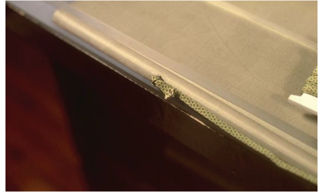
Fig. 28. The second loop covers the metal when it is tightened
