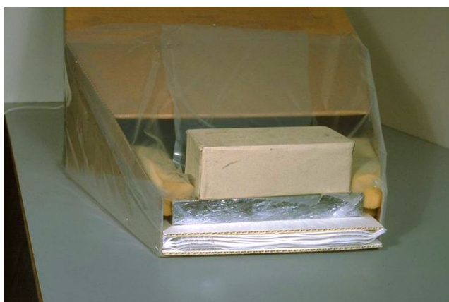
Fig. 7. Polythene sheeting and close-celled foam seal the wind tunnel around the book
