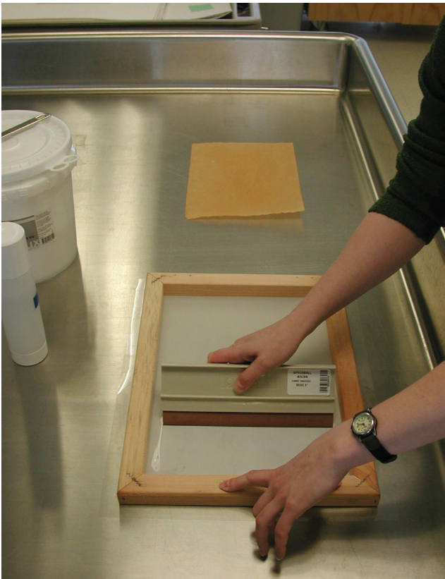
Fig. 1. Squeegeeing through silkscreen onto polyester film
