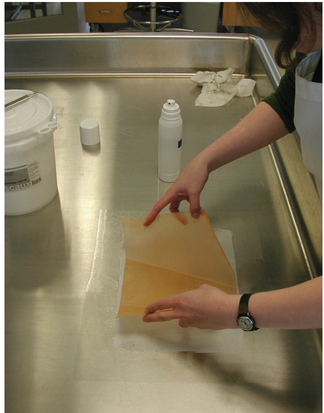
Fig. 2. Dropping wet tissue onto wet adhesive
