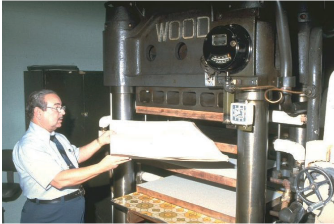
Fig. 2. Wood hydraulic laminating press, NARA
