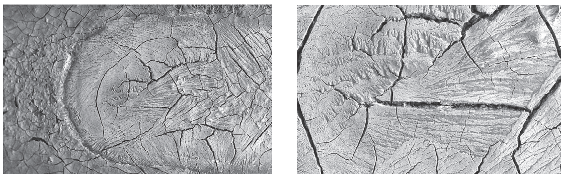
Figs. 8c–d. 1: 1.52: 0.25 (weight ratio of iron (II) sulfate: gallnuts: gum arabic)
