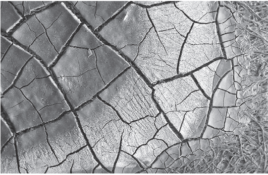
Figs. 9a–b. 1:2.0:0.5 (weight ratio of iron (II) sulfate: gallnuts: gum arabic) after artificial aging by humidity cycling at constant room temperature.
