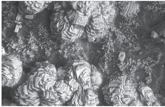
Figs. 9e–f. 1:1.52:0 (weight ratio of iron (II) sulfate: gallnuts: gum arabic) after artificial aging by humidity cycling at elevated temperature.
