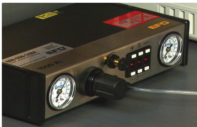
Fig. 1. EFD controller 1500XL fluid dispensing unit with compressed air gauge (at left) and vacuum control gauge at right; regulator valve and program timing controls at center.
