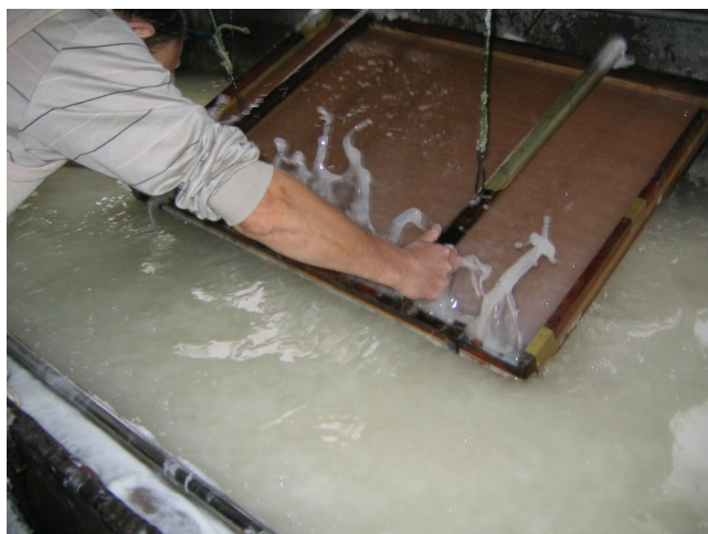
Fig. 14. Scooping fibers onto mold with deckle. Photo courtesy of FIDES.
