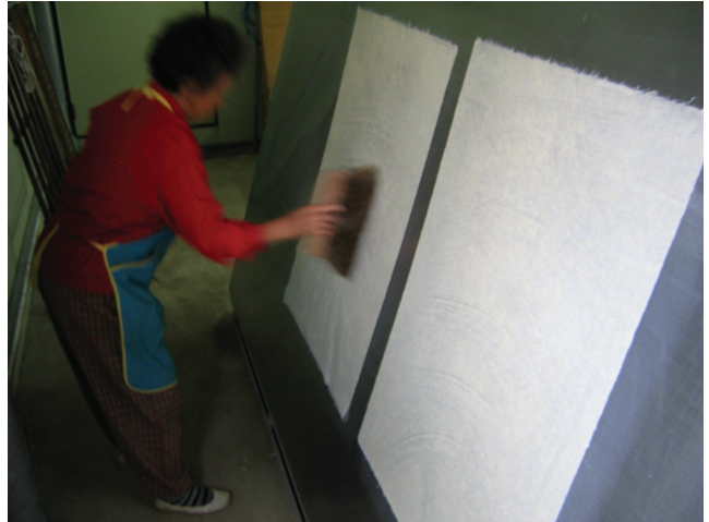
Fig. 20. Drying by brushing individual sheets onto heated stainless steel drum. Photo courtesy of FIDES.
