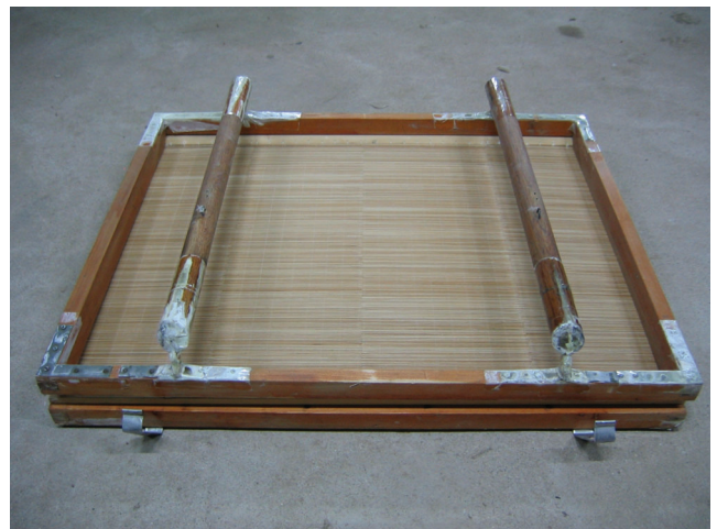
Fig. 13. Mold and deckle for ssangbal method. Photo courtesy of FIDES.
