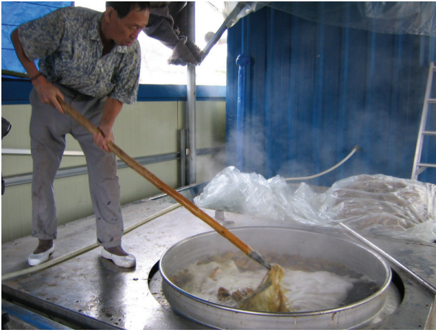
Fig. 3. Cooking white bark with alkali to remove non-cellulosics. Photo courtesy of FIDES.
