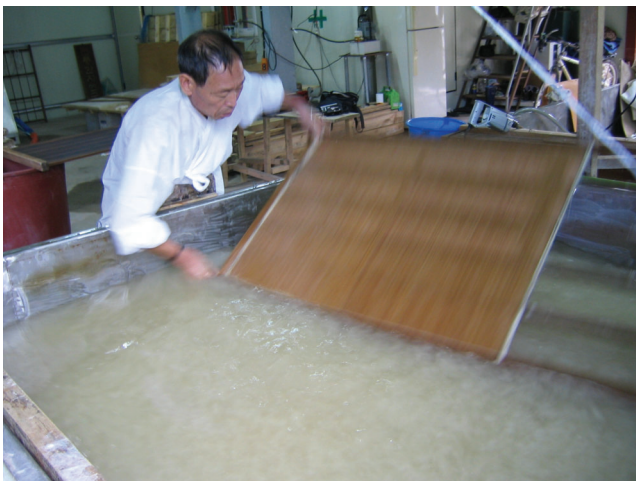
Fig. 12. Dipping the right side of the mold into vat. Photo courtesy of FIDES.
