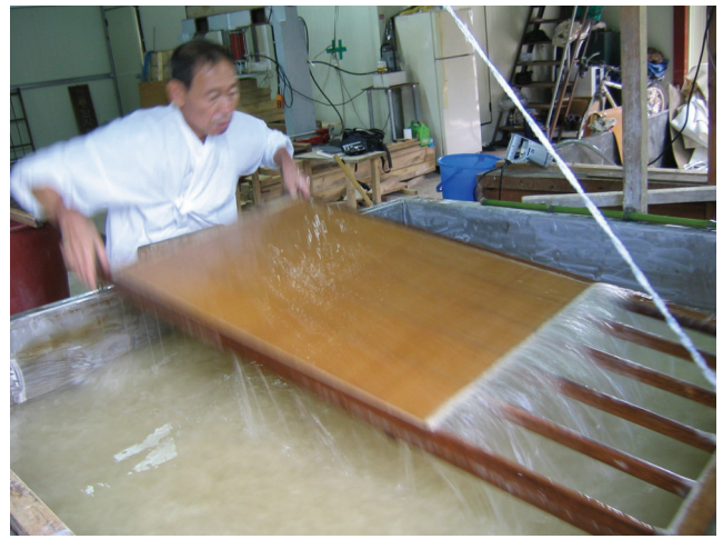
Fig. 9. Fibers flowing off the opposite side of the mold. Photo courtesy of FIDES.
