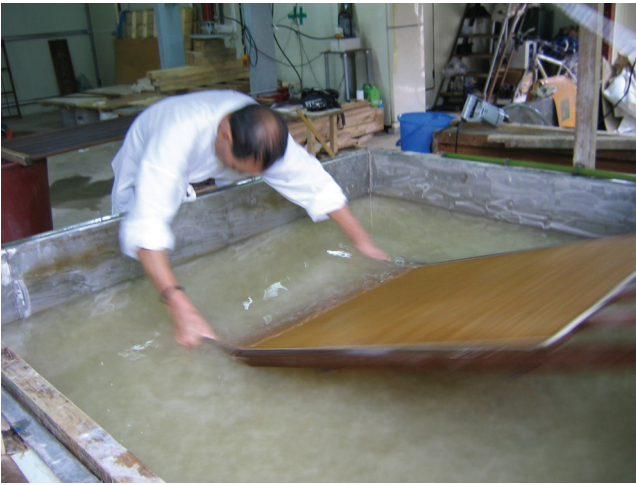
Fig. 8. Initial dip of webal method of sheet forming. Photo courtesy of FIDES.
