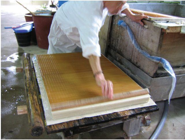
Fig. 17. Sheet is couched onto post of wet sheets. Photo courtesy of FIDES.
