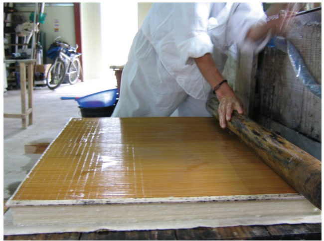
Fig. 18. Rolling log across post of wet sheets to remove bubbles. Photo courtesy of FIDES.
