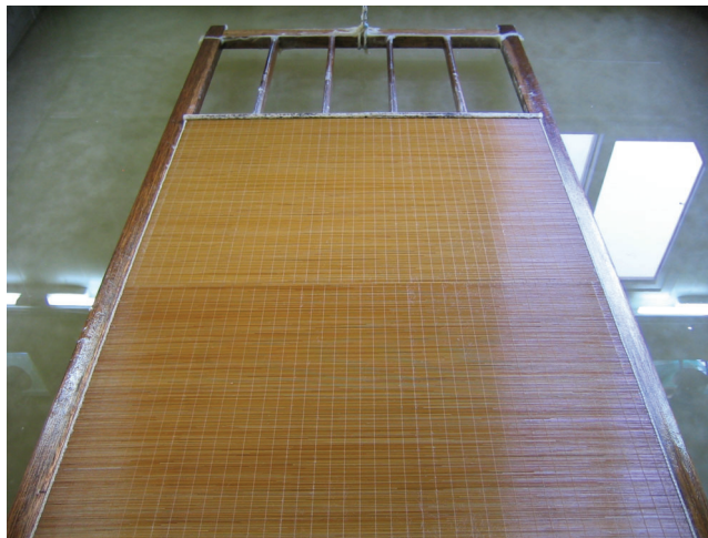
Fig. 2. Mold and screen for webal method. Photo courtesy of FIDES.
