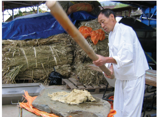
Fig. 6. Traditional beating method with stick. Photo courtesy of FIDES.
