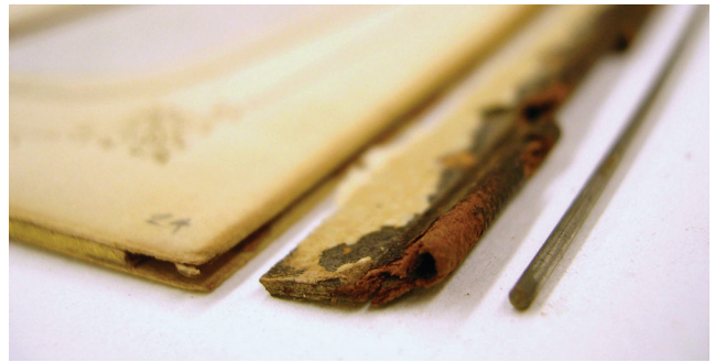
Fig. 9. Disassembled leaf, loop hinge, and rod
