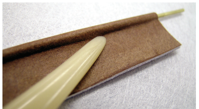
Fig. 12. Dyed Japanese paper and cotton flannel laminate: final shaping and burnishing
