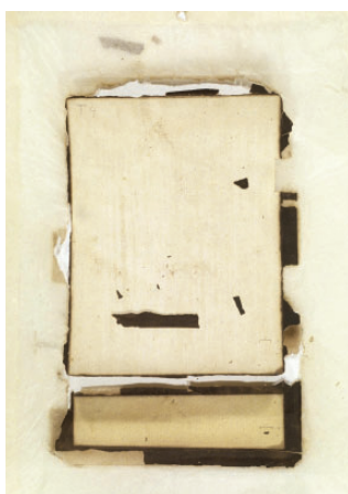
Fig. 7. Paper T4, deacidification with calcium bicarbonate, lining with wheat-starch paste, after aging.
