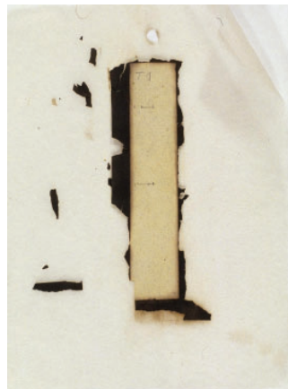
Fig. 4. Paper T1, nonaqueous deacidification, lining with Klucel G, after aging.
