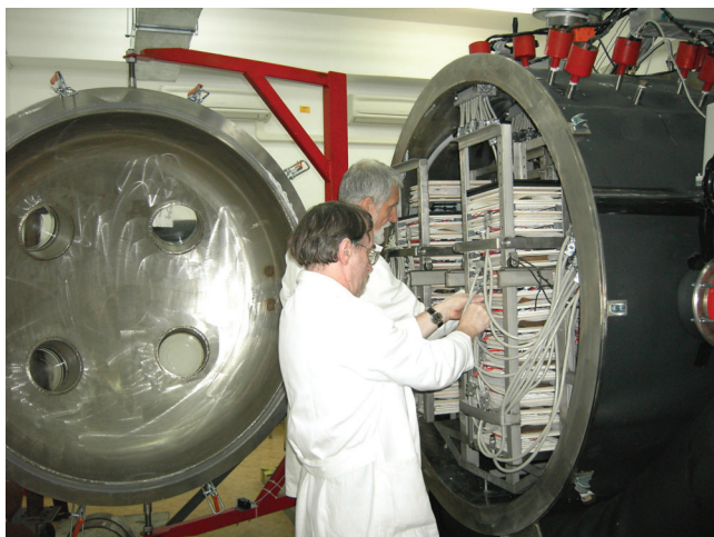
Fig. 3. Connecting cables to the heating tiles
