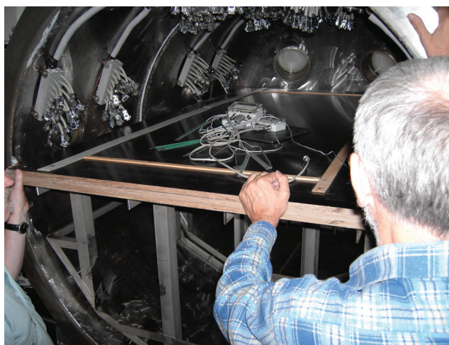
Fig. 6. Preparing the chamber for the drying of large-format documents
