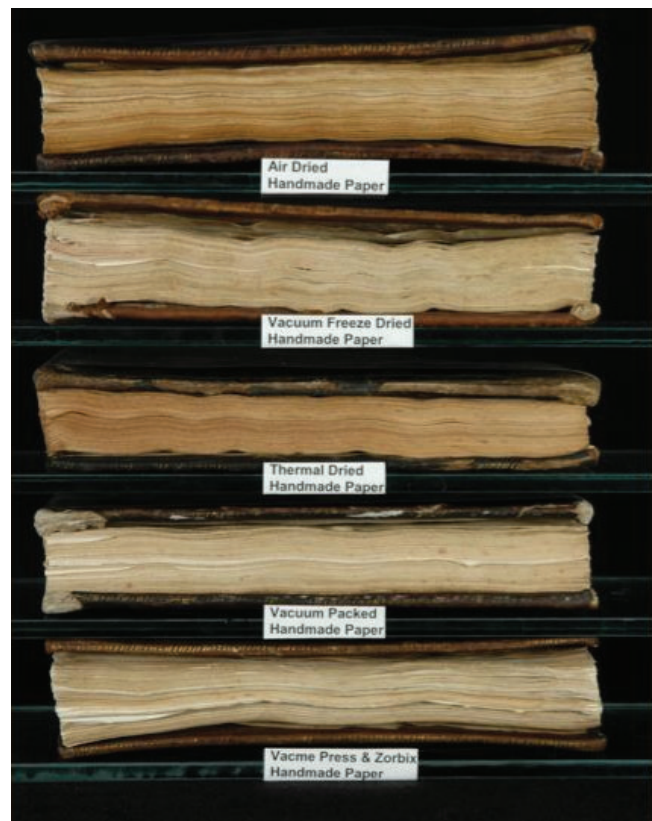
Fig. 17. Comparison of physical cockling in handmade paper
