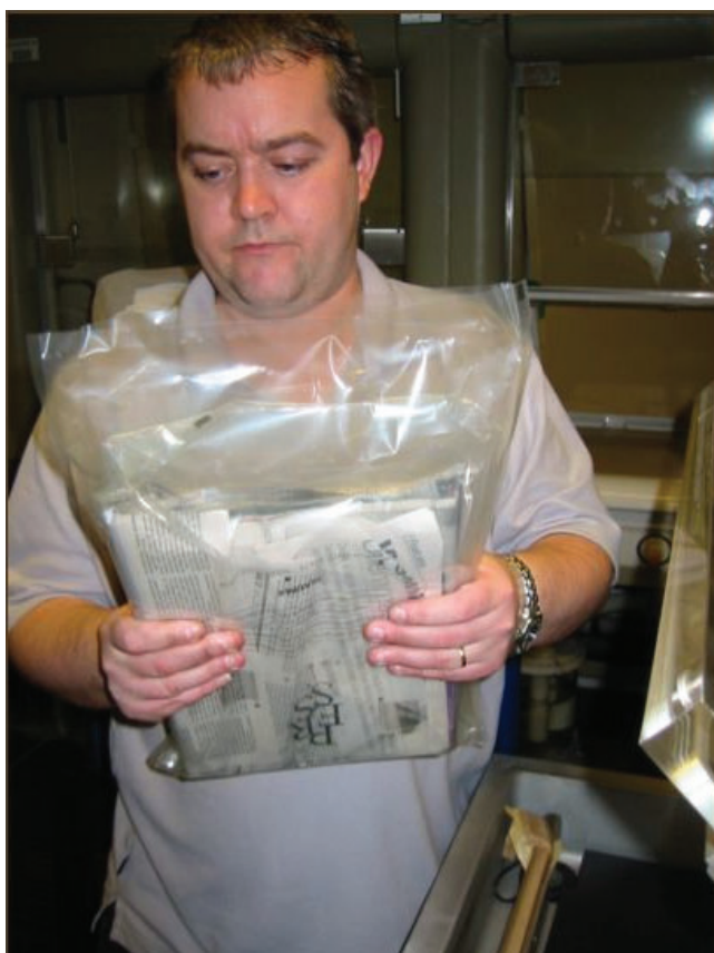
Fig. 8. Interleaved book in pouch prepared for vacuum packing, British Library
