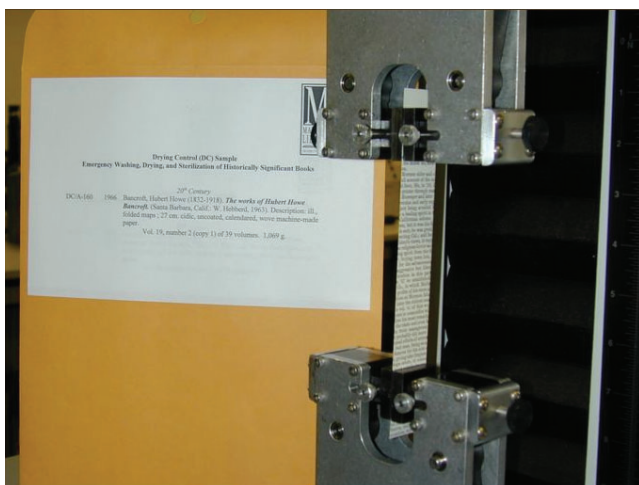
Fig. 13. Analytical testing: tensile test, Applied Paper Technology, Inc
