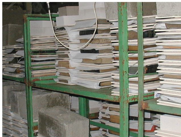
Fig. 7. Books stacked between unglazed ceramic tiles in kiln, Czech Republic
