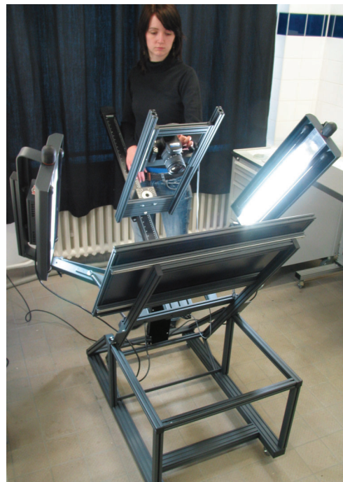
Fig. 3. Digital photography copy stand constructed by Dipl. –Ing. Manfred Meyer (Graz, Austria) as a custom design for the Kupferstichkabinett; conservation intern Josephine Werthman pictured.
