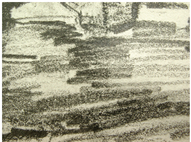
Fig. 3. Image of brush application over graphite showing left side saturated and right side uncoated. (Photo Joan Weir)
