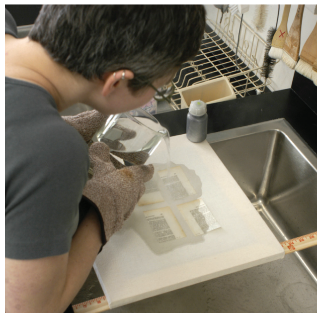
Fig. 5. Pouring boiling water over the samples from 1836
