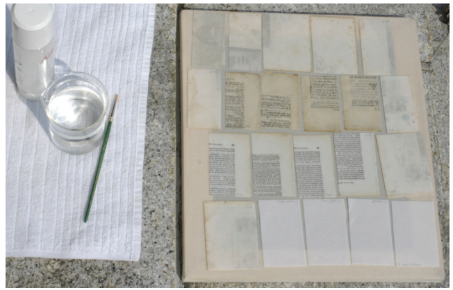
Fig. 7. Sun bleaching outside on the muslin washing frame
