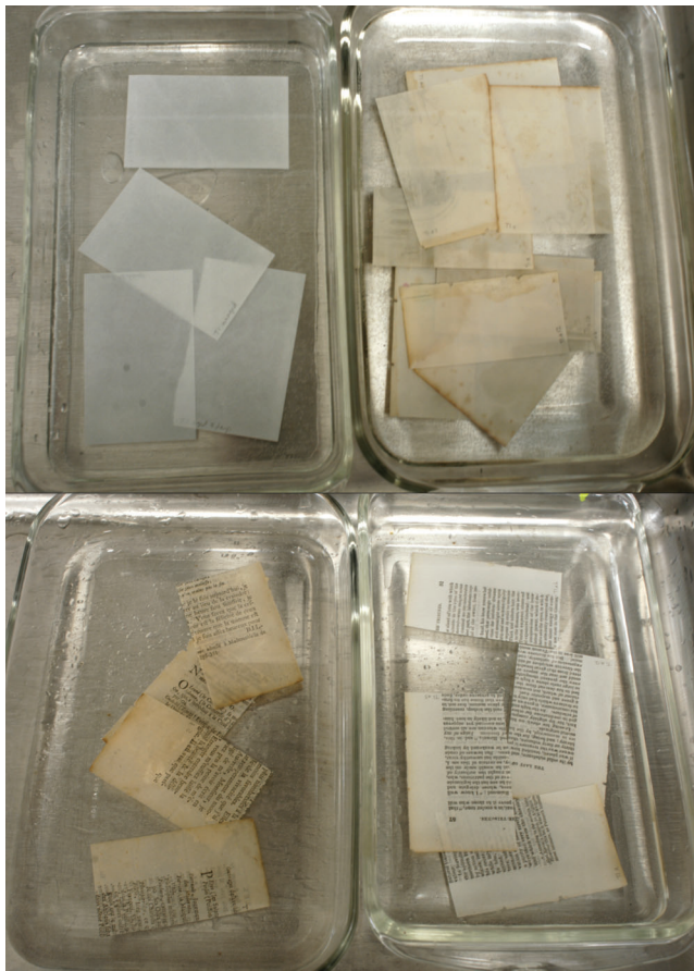
Fig. 6. Paper samples soaking for twenty-nine hours in tap water
