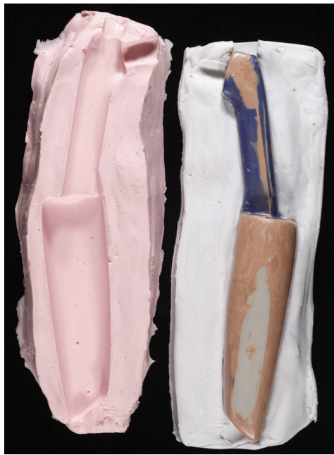
Fig. 5. Cured silicone rubber mold with prototype
