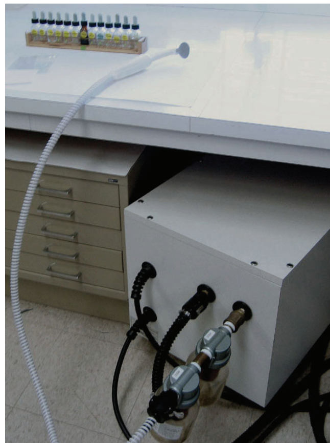
Fig. 7. Hand-held suction device attached to a positive displacement vacuum pump
