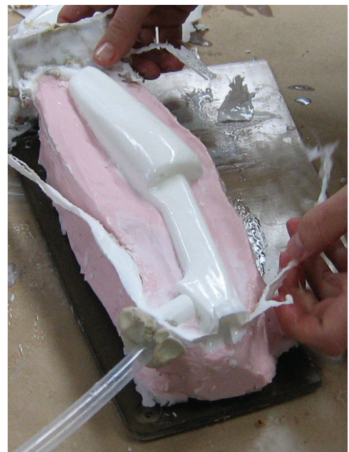
Fig. 6. Handle cast in polyurethane resin
