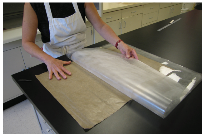
Fig. 14. When the paper is dry, peel off the Mylar support from the back
