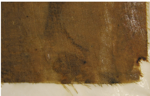
Fig. 2. Verso, detail of the frayed edges of a large, varnished map impregnated with SCMC. Phelps & Ensign's Travellers' Guide, and Map of the United States, 1837, 1840 . Intaglio on wove paper, hand-colored. 0.745 x 1.05 m, Map Library, University of Michigan Library, no catalog number.
