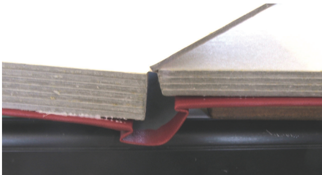
Fig. 15. Detail showing restricted opening and pastedowns becoming detached
