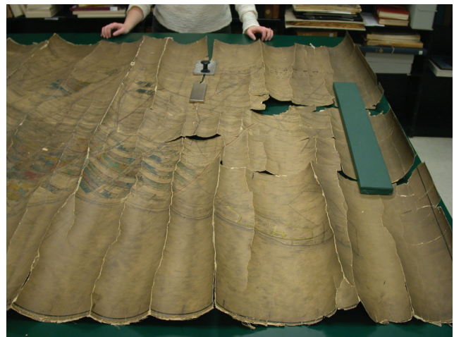
Fig. 7. A hardback map showing tears, losses, and a regular pattern of creases
