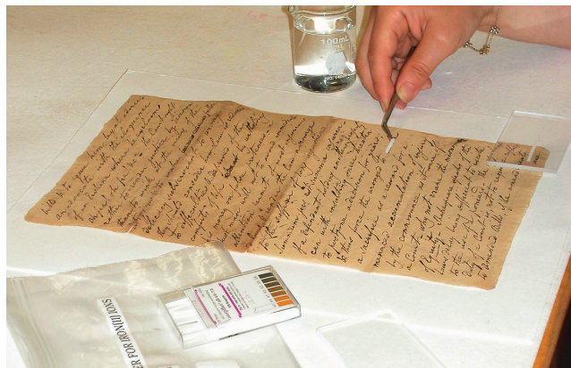
Fig. 1. Testing for presence of iron (II) ions
