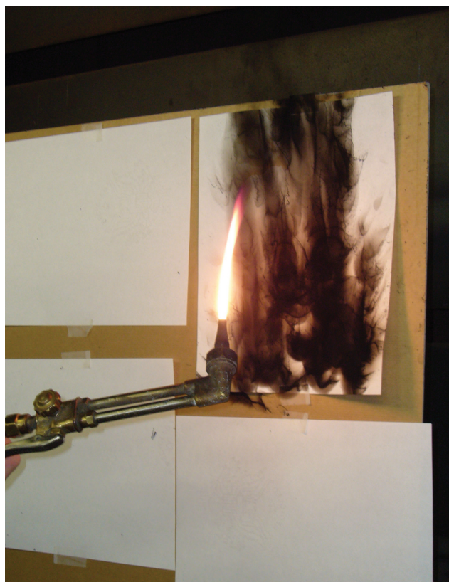
Fig. 3. Making soot samples with oxy-acetylene welding torch
