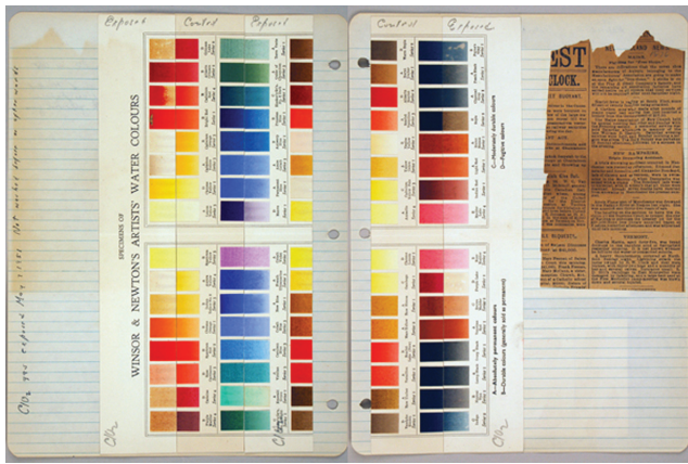
Fig. 6. Pages from Gettens's bleaching notebook: chlorine dioxide bleaching tests on Winsor & Newton's Artists' Water Colours, May 7, 1951
