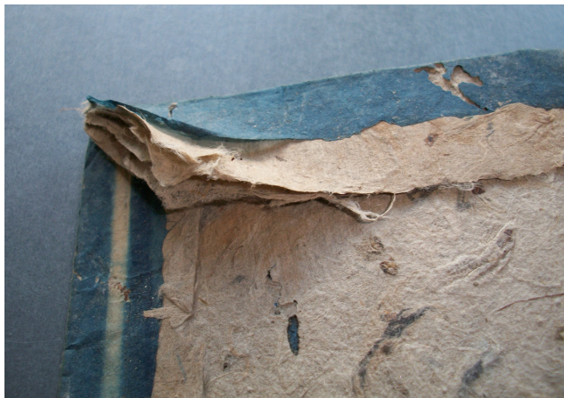
Fig. 4. Example of a book cover construction showing the laminated layers of recycled paper and a sheet of dyed paper and turn-ins
