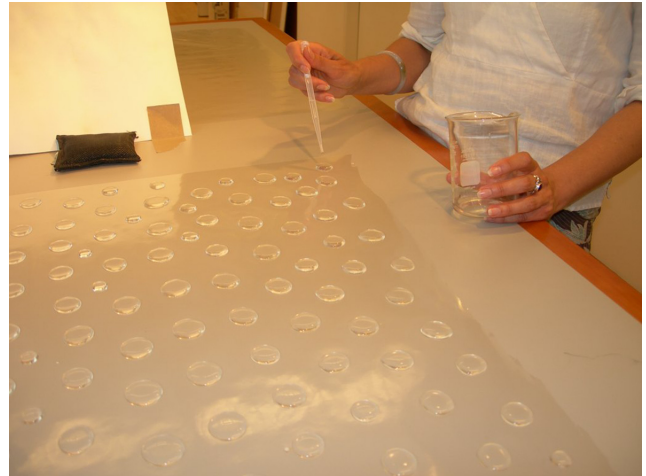
Fig. 13. Disposal pipettes dispensing the isinglass liquid into disk shapes to be dehydrated and stored for future use
