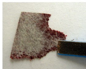
Fig. 9. Cast composite fill is sanded to expose the cast film along the edge.
