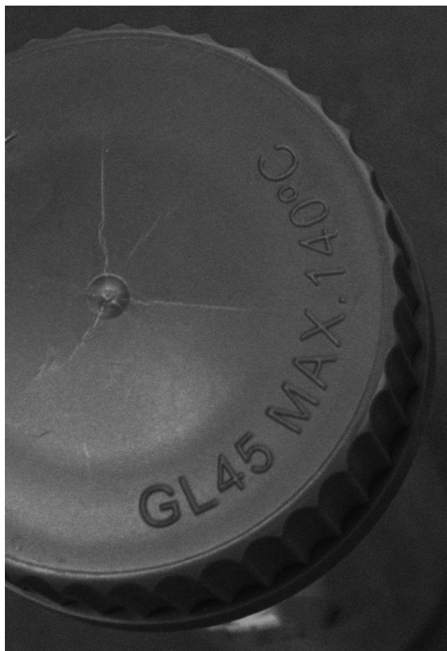
Fig. 4. Failed accelerated aging vessel showing fractures on the screw cap
