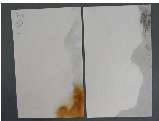
Fig. 2. Alum rosin sized paper, image taken at day 19. Similar quantities of mold growth were seen on untreated sample on left and Bookkeeper treated sample on right. Growth on untreated samples of this paper type was slightly greater in quantity and much more colorful. Tidelines are slightly more pronounced on Bookkeeper treated samples
