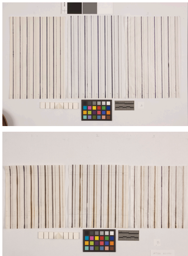
Figs. 22–23. Samples before aging, top, and after post-treatment aging, showing brown haloing around inks containing sugar, bottom
