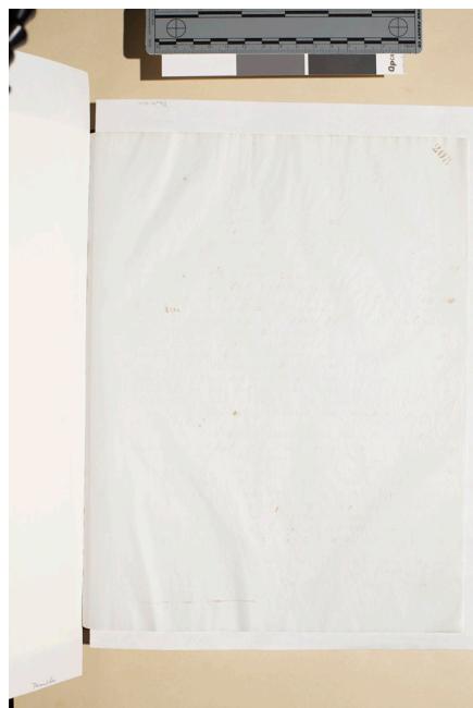
Figs. 24–26. Baird copying book, volume 71, page 118. Example of Baird copying book digitization using interleaving, a ring flash, and image processing to increase legibility and decrease distraction from translucency, distortion, and surface details. Left, page photographed in reflected light with a ring flash and no interleaving and no image processing. Middle, page photographed in reflected light using a ring flash with an interleaving sheet and no image processing. Right, page photographed in reflected light using a ring flash with an interleaving sheet and minimal image processing using Digital Photo Professional
