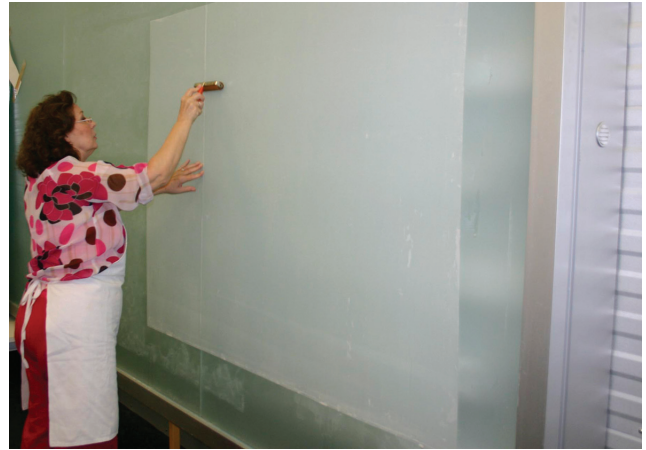
Fig. 13. A pasted-out sheet of Terylene being smoothed onto the glass surface of the light wall
