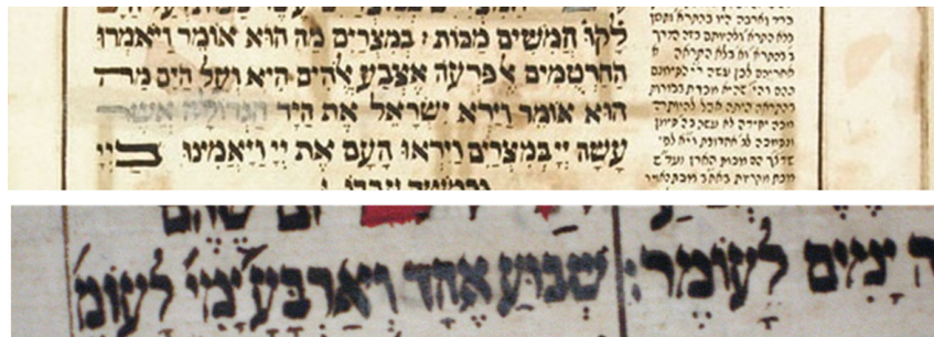
Fig. 3. 1987 repair using Japanese tissue (top) and most recent repairs using the gelatin-coated Berlin tissue (bottom) (Courtesy of Library and Archives Canada)
