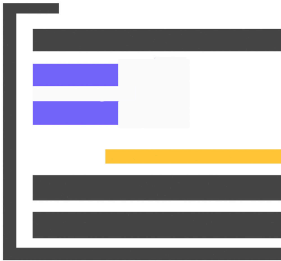
Fig. 8. Diagram of the layers of the housing package for Martin's Portrait of Garrison Wright . From top to bottom: glazing, spacers, pastel, rigid backing boards, and barrier film that wraps around to the front of the glazing
