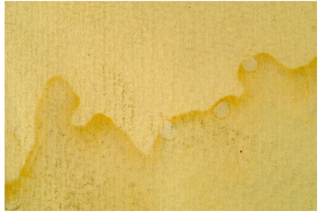
Fig. 7. The tide line with local tests using conductivity-adjusted agarose pellets. From left to right: 1,000 \mu\text{S}/\text{cm} , 5,000 \mu\text{S}/\text{cm} , and 10,000 \mu\text{S}/\text{cm}
