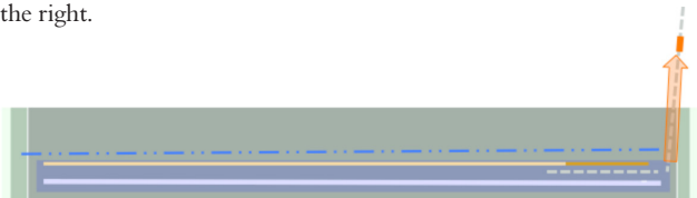
Fig. 30. The object is positioned on the blotter with the stain over the wick. A sheet of polyester film rests over the item, and the solvent eventually evaporates up the wick.
