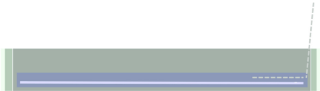
Fig. 29. Tray of polyester film containing blotter and sufficient solvent to saturate the blotter. The creased filter-paper wick is seen at the right.
