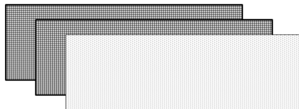
Fig. 26. The three layers of material to be placed inside the plastic channel: the layers allow the passage of air through the plastic to the suction device.
