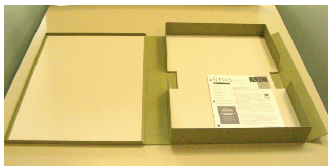
Fig. 3. The completed box includes a bottom tray with hand notches, lined with paper-covered Volar foam, and a shallow, lightweight top tray that secures the fore-edge flap, thus stabilizing and sealing the box from dust, etc.
