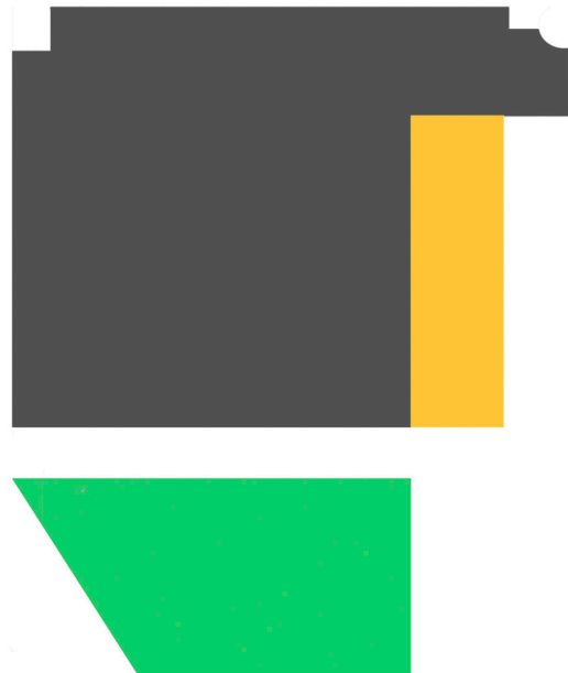
Fig. 9. Diagram of frame profile and alteration for Martin's Portrait of Garrison Wright . The section below the lip of the frame was removed and a wooden buildup was added to the back.
