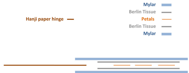
Fig. 20. Diagram of encapsulation assembly. The Berlin tissue is from Gangolf Ulbricht in Germany.
