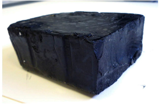
Fig. 1. Half of an oilstick brick, 10.6 x 8.89 x 4.45 cm (4 x 3 ½ x 1 ¾ in.), made by melting oilsticks, adding linseed oil, and cooling in a mold
