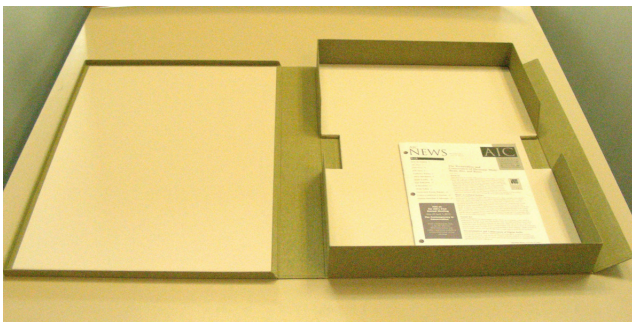
Fig. 3. The completed box includes a bottom tray with hand notches, lined with paper-covered Volar foam, and a shallow, lightweight top tray that secures the fore-edge flap, thus stabilizing and sealing the box from dust, etc.
