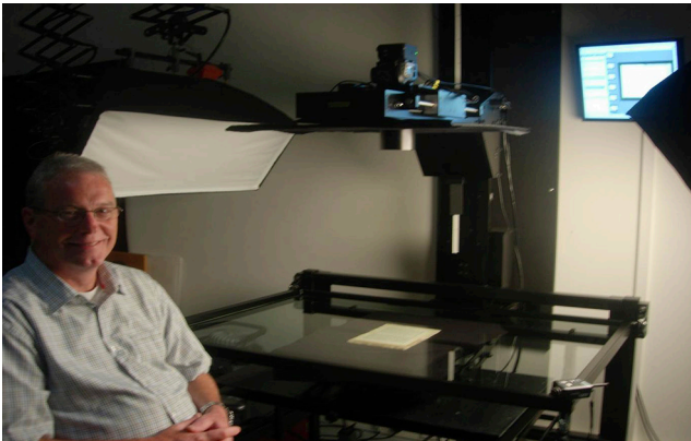
Fig. 18. Guardian Copy Stand System: 180 degree opening.
