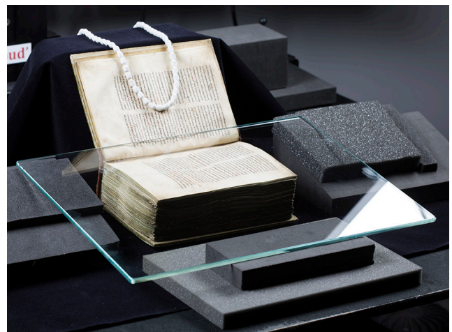
Fig. 16. A regular copy stand with 90–110 degree opening.
