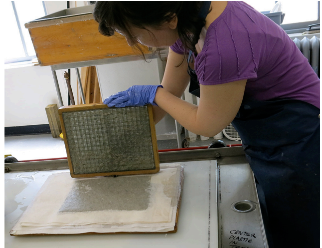
Fig. 11. A sheet formed on the mould's screen transferred onto a pile of previously made paper interleaved with synthetic fabric.
