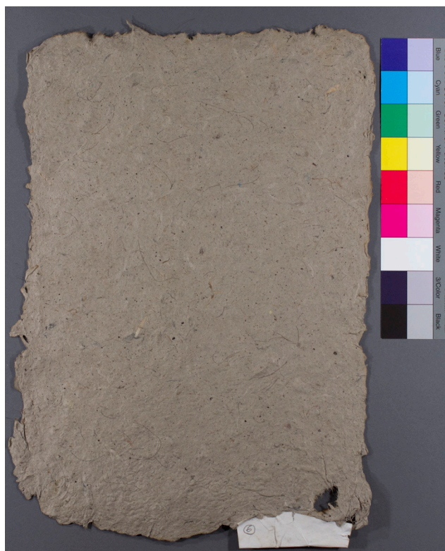
Fig. 16. Paper sample made in Trial 3, which used uncooked waste paper.
