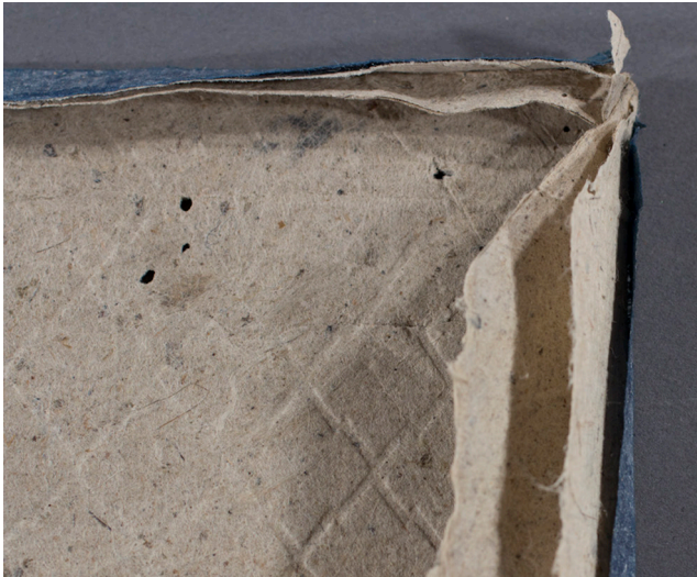
Fig. 4. Example of a book cover construction showing two laminated layers of recycled paper and a sheet of dyed paper.
