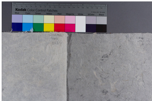
Fig. 15. Paper samples made in Trial 2, washed and beaten once. The paper on the right used uncooked waste paper; the left used waste paper cooked with wood ash.
