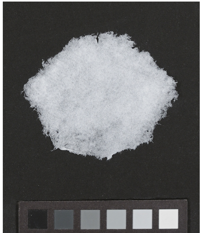
Figs. 2a–2b. In these two comparative images, it is possible to observe how a 0.06 mm paper made of 100% flax fibers (below) is more opaque than a 0.06 mm paper made of 100% cotton fibers (above).
