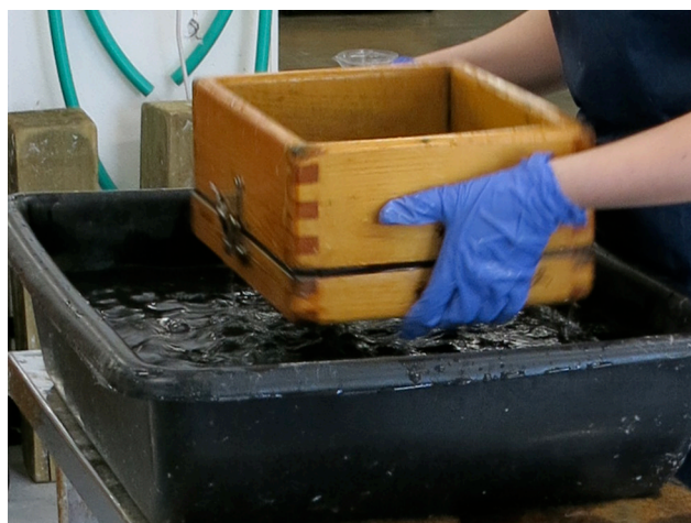
Fig. 10. Papermaking mould consisting of upper screen frame and lower box.
