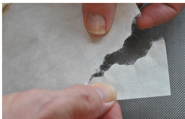
Fig. 7. Dry-tearing of perforated paper.
