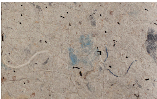
Fig. 6. Recycled paper book cover exhibiting contained impurities, such as pieces of fabric plants, paper, dust, and hairs.
