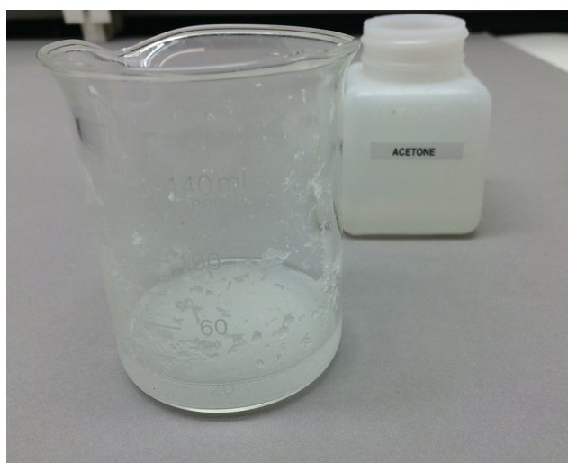
Fig. 2. Acetone will partially dissolve Plexiglas and will be semi-transparent and milky-white in color.
