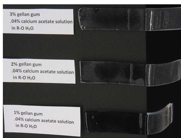
Fig. 4. Comparison of rigidity of gellan gum concentrations incorporating calcium acetate.
