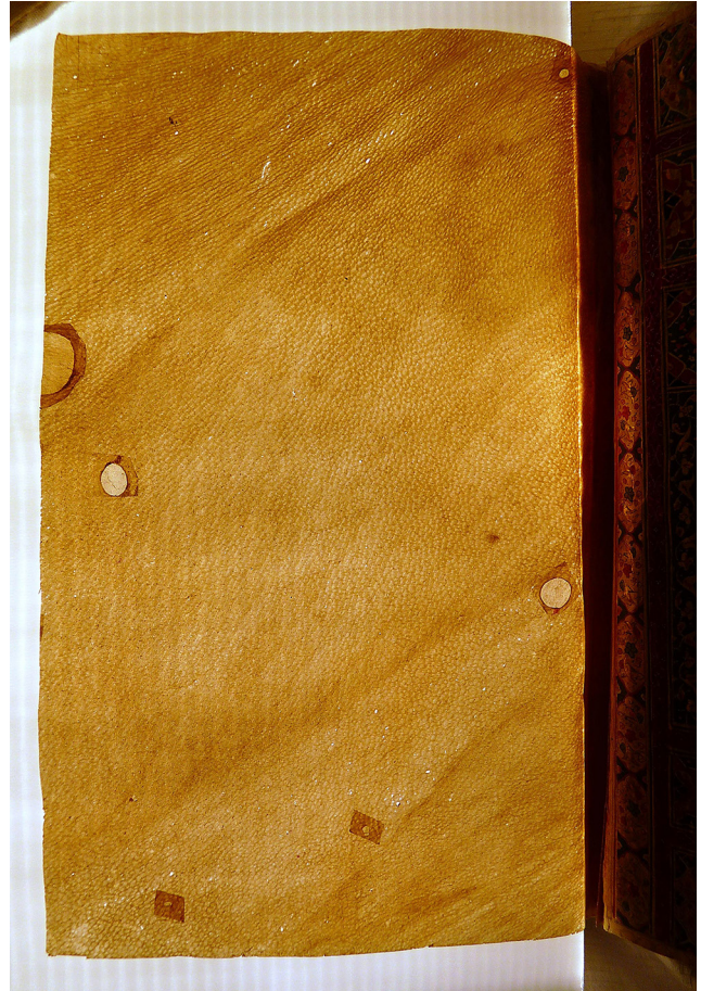
Fig. 5. Copy of the Qur'an, acc.no.MS.366. MIAQ, with transmitted light, the interleaf shows characteristic marks probably caused by the action of a blade; the holes were mended with a similar type of skin.
