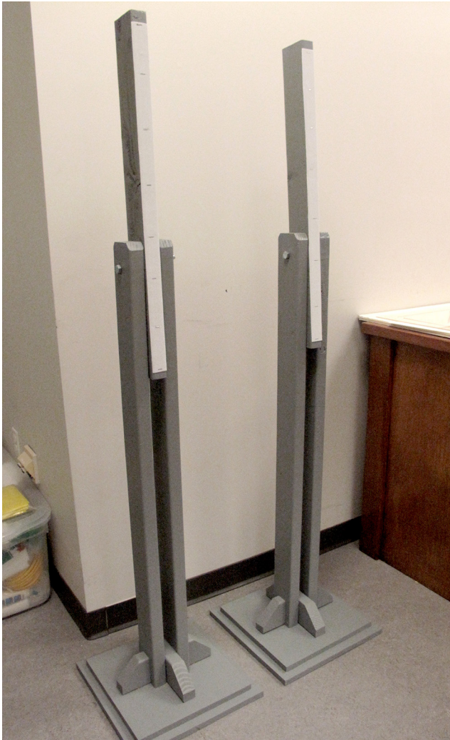
Fig. 9. One of the floor stands, constructed of common lumber and industrial Velcro.
