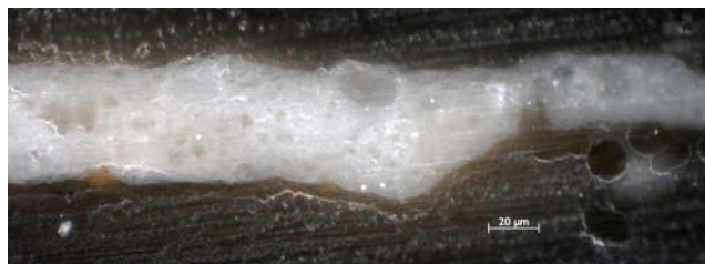
Fig. 4. 50× dark-field image of a cross section taken from the lower tacking margin of The Man with the Dog . The sizing and ground layers are visible. The uppermost layer is adhesive from gummed tape or a paper dust cover.
