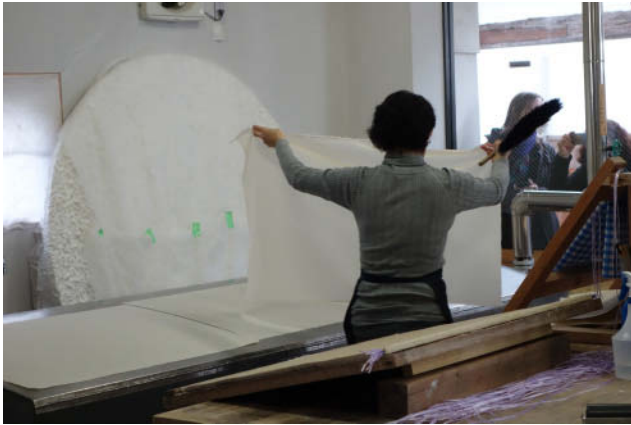
Fig. 13. Mrs. Hamada separates sheets of paper from the post. She is holding the brush used to apply the sheet to the drying surface, which is a rotating, heated stainless steel drum behind her. Hamada Washi, Kochi Prefecture. Credit: Jacinta Johnson.
