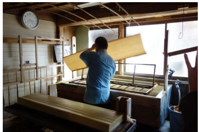
Fig. 12. Mr. Fukunishi making udagami with the nagashizuki method. The organization of the studio and the tools used in the step depicted here include the vat; the bamboo struts over the vat; the hinged frame and deckle called the keta ; the removable, flexible screen called the su ; the post behind the papermaker with the wooden guides; and fishing wire placed along the edge closest to the papermaker to assist in sheet separation. Fukunishi Studio, Nara Prefecture. Credit: Jacinta Johnson.
