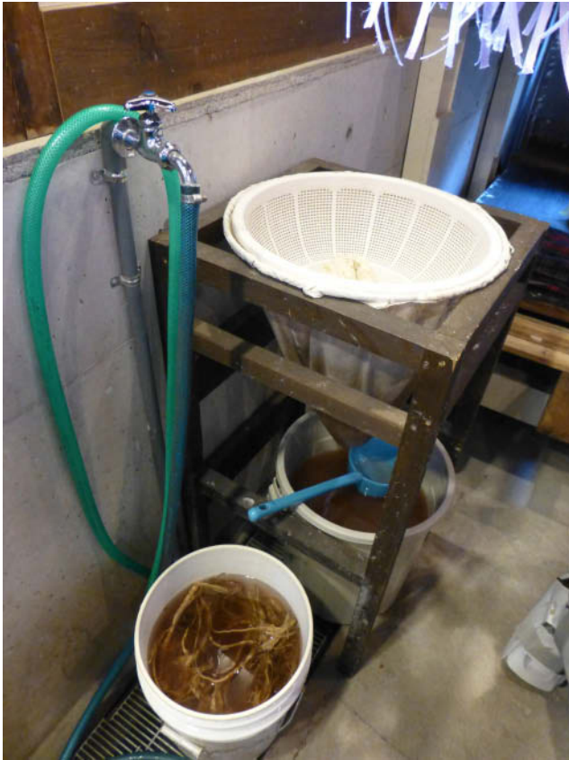
Fig. 9. Neri dispersion agent extracted from the tororo-aoi root by crushing and soaking in water. Neri is scooped from the bucket and passed through a strainer before it is added to the vat.
