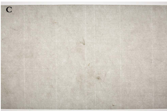
Fig. 22c. Detail of a paper made with a bamboo screen in transmitted light. The narrower chain lines, double chain lines, and finer laid lines are visible. Credit: Matthew Hamilton.
