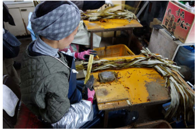
Fig. 20. Papermakers retain the green nazekawa layer of the kozo bark when making sekishu-banshi . This layer is composed mainly of hemicellulose and imparts unique characteristics of the paper. Sekishu Kubota Studio, Shimane Prefecture. Credit: Jacinta Johnson.
