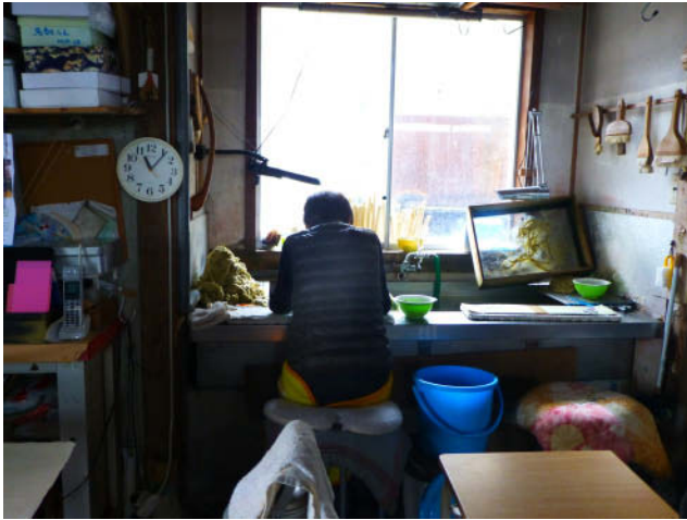
Fig. 6. Mrs. Kubota removing blemishes from cooked bark in the chiritori process. Sekishu Kubota Studio, Shimane Prefecture.
