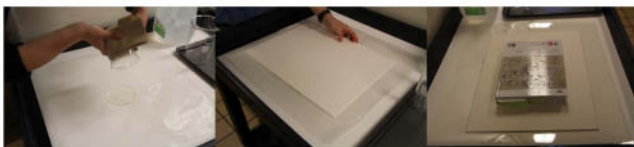
Fig. 5. Steps to make agarose film, from left to right: pour the hot agarose on a polyester sheet; place on top another polyester sheet and a board; apply weight on top (around 2 kg/4.4 lbs.).
