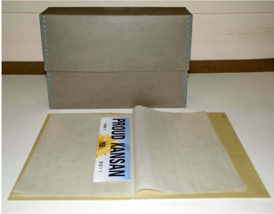
Fig. 6. Bumper sticker within folded piece of silicone release paper, placed within a standard alkaline folder. Credit: Whitney Baker.
