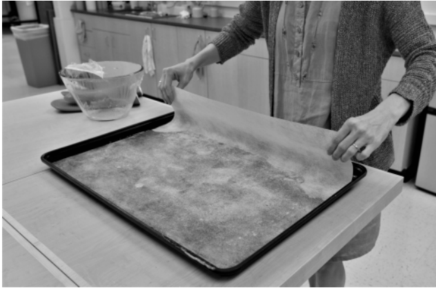
Fig. 5. Leave a tab of spun polyester at one side to ease lifting so that the gellan gum is not pinched or damaged.
