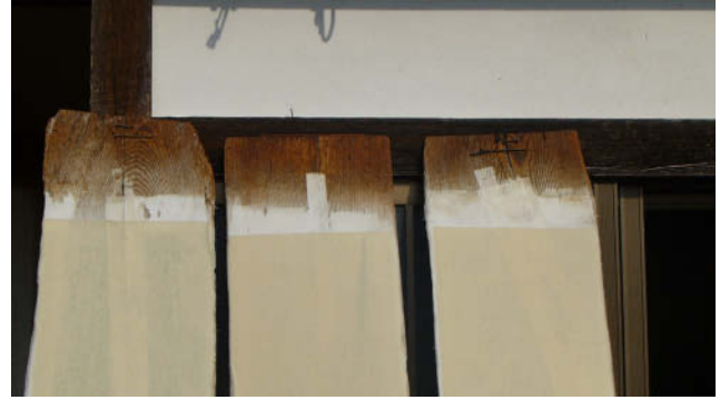
Fig. 15. Papermakers greatly value their drying boards as is evident by the repairs made with metal staples and kozo patches to secure splits and cracks. These boards used at the Fukunishi Studio in Nara Prefecture are 300-year-old pine heirloom drying boards. Fukunishi Studio, Nara Prefecture.
