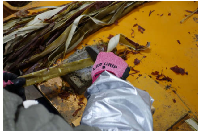
Fig. 4. Scraping unwanted layers of outer bark with a knife. Sekishu Kubota Studio, Shimane Prefecture. Credit: Jacinta Johnson.
