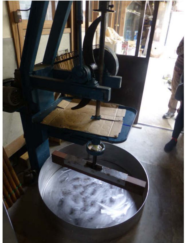
Fig. 8. A mechanical beater used in place of hand beating paper fibers. In some studios hand-beaten fibers are then further beaten using the mechanical beater. Fukunishi Studio, Nara Prefecture.
