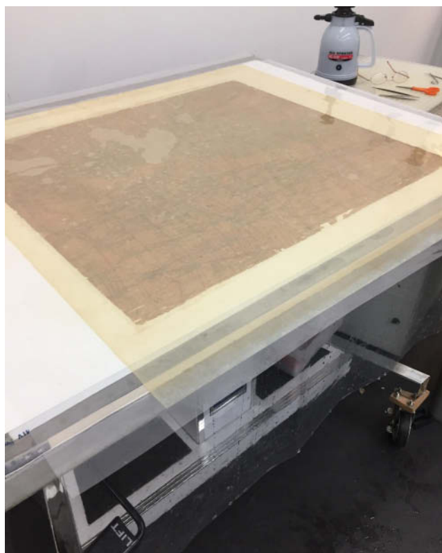
Fig. 4. Lining directly on suction table. One quarter of J.B. Beers & Co., Kings and Queens Counties, New York , 1886, NYPL Map Division 16-5970.
