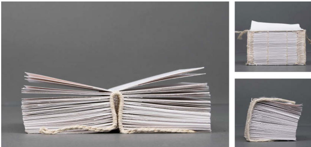
Fig. 10. Opening characteristics of a model sewn with unsupported link stitch.
