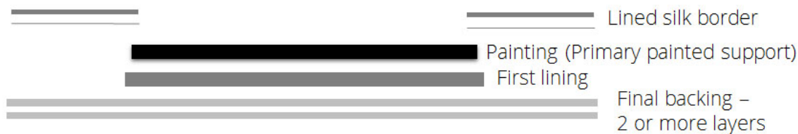
Fig. 4. Cross sectional view of laminate structure of a standard mounted Chinese painting
