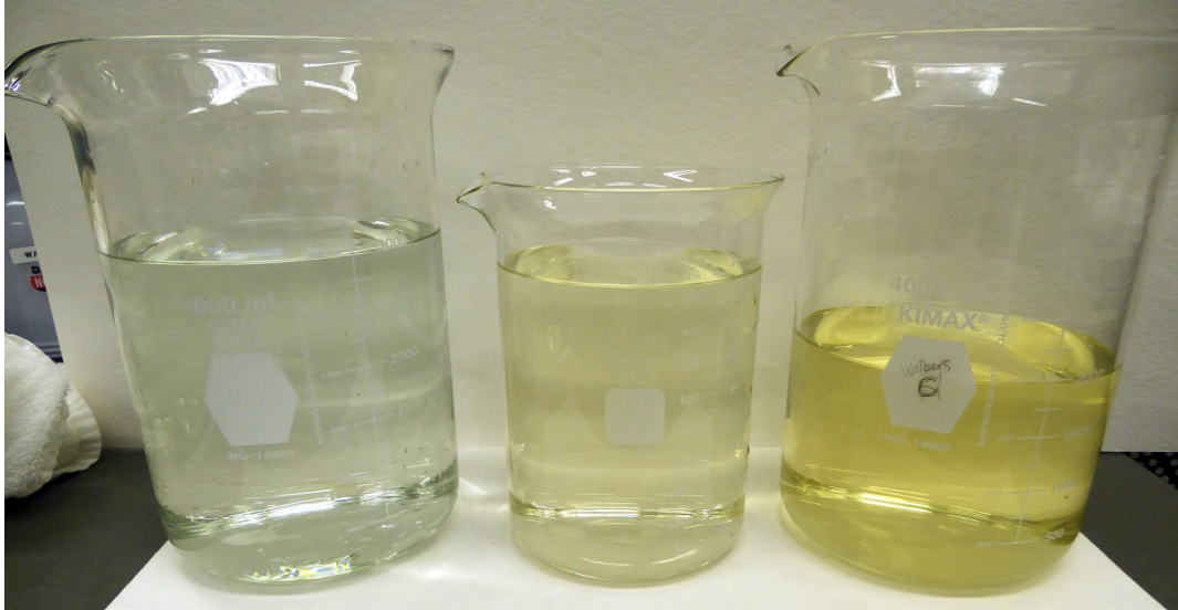
Fig. 7. Water collected from Solution D bath (right), first rinse bath (center), and second rinse bath (left).
