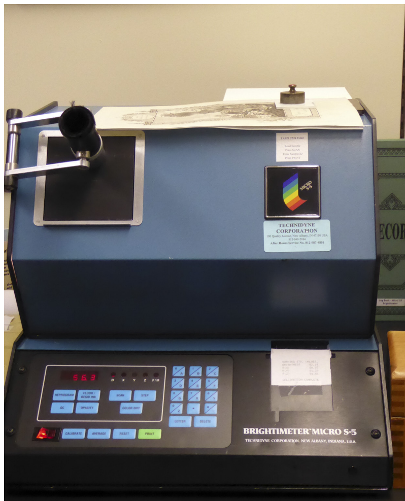
Fig. 2. Brightmeter measurement of Print 2.2.
