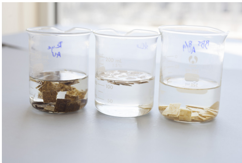
Fig. 7 & 8. Cold extraction pH testing of various paper samples
