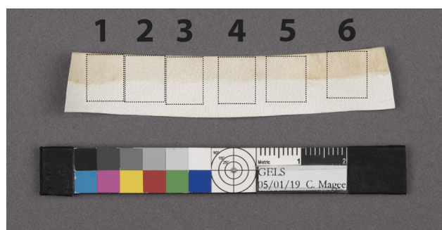
Fig. 13. The efficacy of the six experimental gels (see table 1) were tested in the reduction of an artificially created tide line on a piece of modern goatskin parchment. Image courtesy of the Walters Art Museum.
