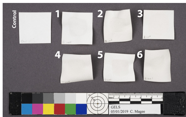
Fig. 14. Squares of modern goatskin parchment were exposed to the six experimental gels and artificially aged in an oven. The control sample was not exposed to a gel. Image courtesy of the Walters Art Museum.
