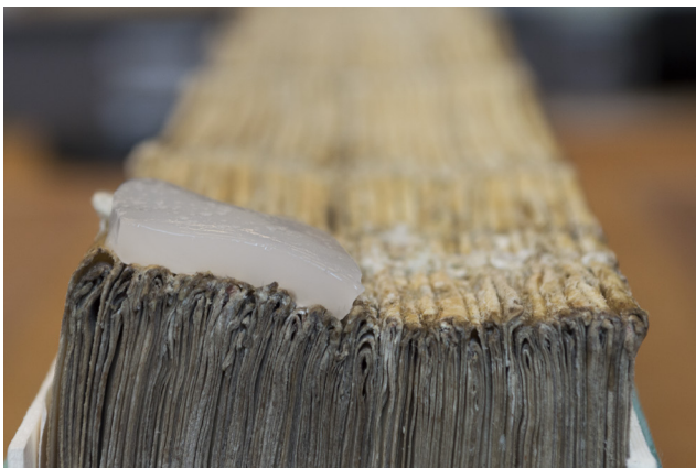
Fig. 10. The ability of HAGG to conform to the uneven book spine was instrumental to the success of the gel.
